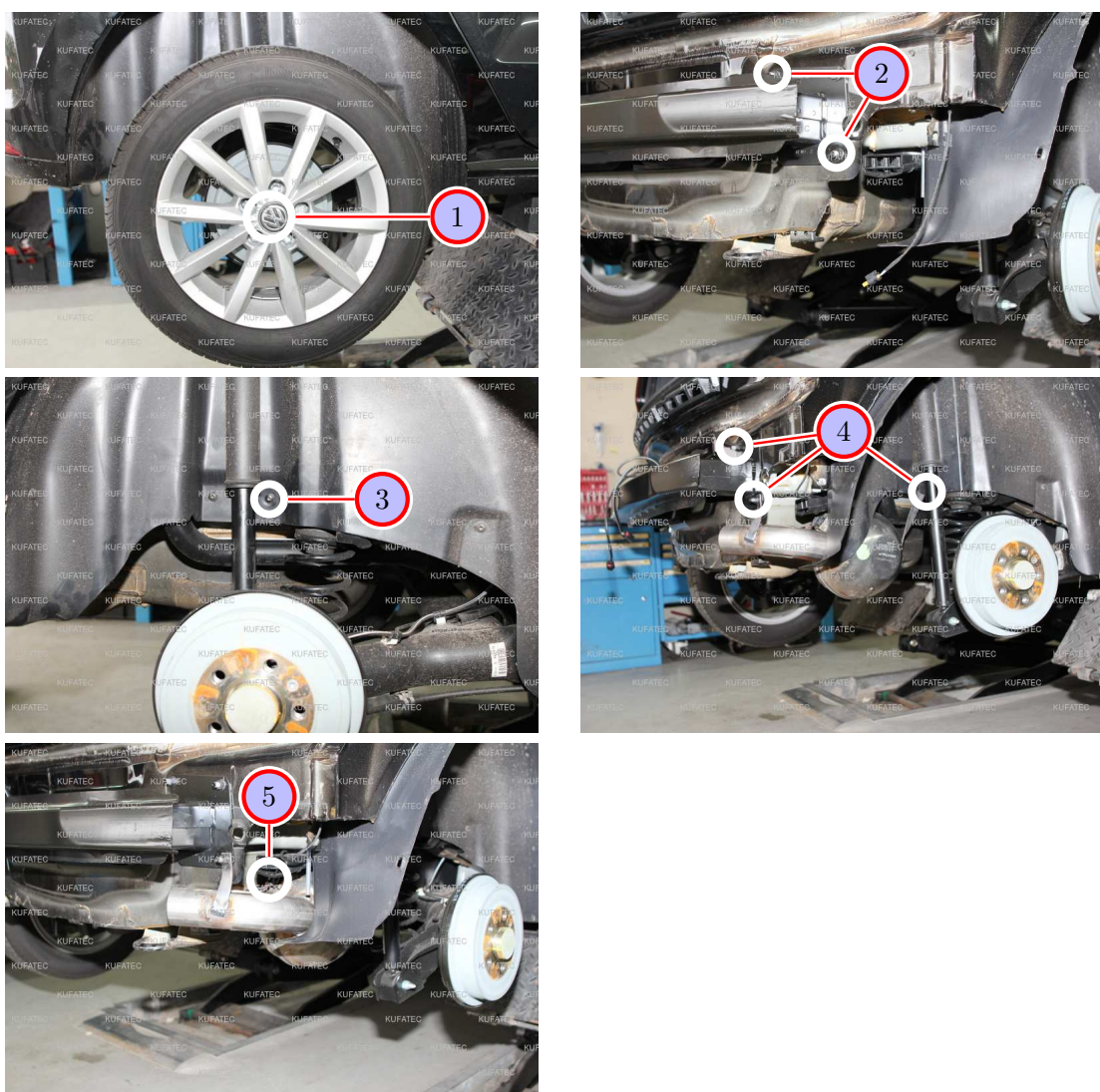
Figure 12: Installation sound generator
